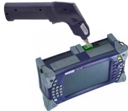
Figure 3: OTDR Port Inspection
